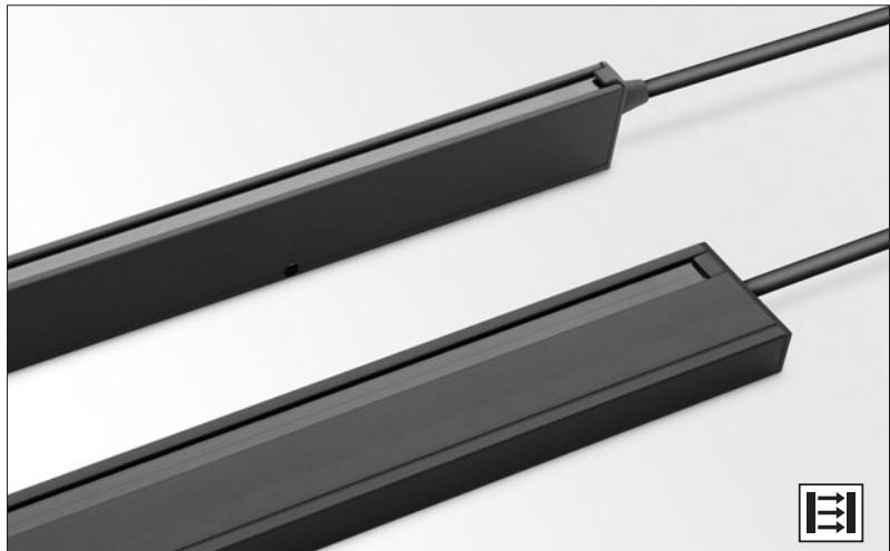
The SG 14 light curtain system consists of a self-contained transmitter detector, SGT and receiver detector, SGR, which are to be positioned opposite of each other. The detectors are housed in a sturdy aluminium profile available in a slim line design (12 x 30 mm) or a leading edge design (38,4 x 14 mm).
