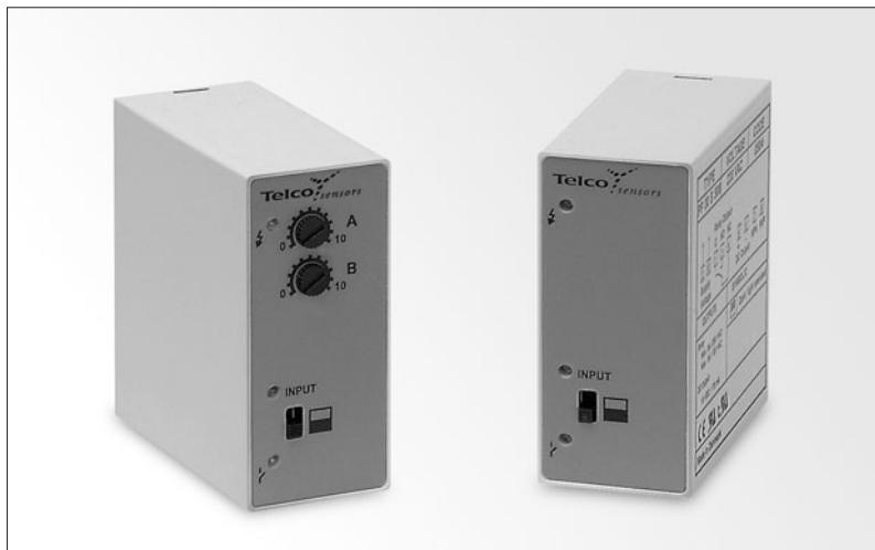
The PP 00 is intended to be used in conjunction with a Spacemaster, SpacePak or SpaceGuard system, where a DC supply voltage is not available and where a relay output is required. This power pack series provides a fixed 15 V dc output voltage, available with or without an adjustable 0-10 sec on/off time delay. Light or dark function is switch selectable.
