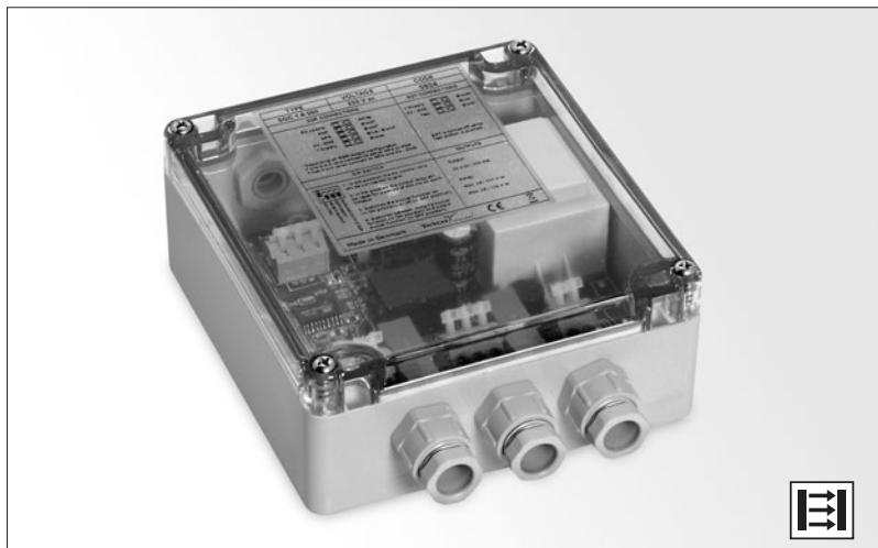
The SGC 1 is intended to be used in conjunction with the SG 1, SG 2, SG 10 or SG 14 self-contained light curtain series, where a DC supply voltage is not available and where an electromechanical relay output is required. The controller series is supplied with a fixed 24 V dc output voltage. Light or dark function and receiver control function is switch selectable.
