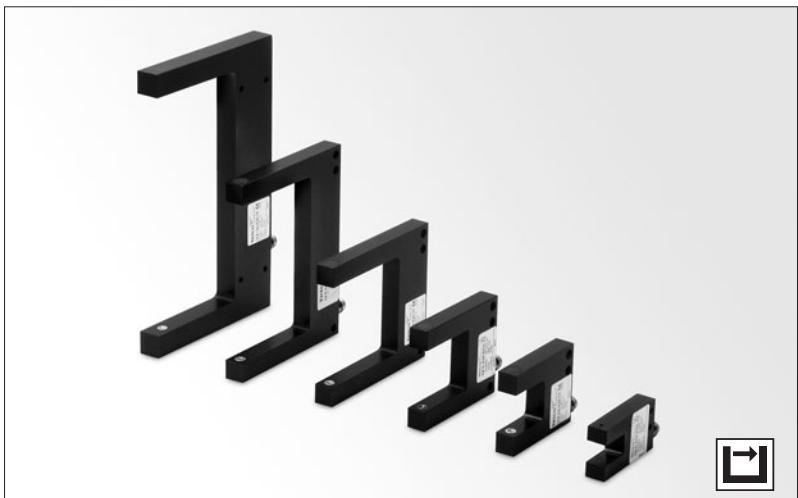
The OFS series consists of self-contained optical fork sensors that are housed in a durable, U-shaped aluminium housing which operates in thru-beam mode, available with infrared (OFS), visible red (OFSR) or high power infrared (OFSH) light source. The series is available with a wide variety of fork opening widths, ranging from 2 mm to 220 mm.
