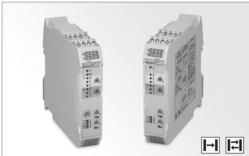
The PAB 20 is a 2-channel, multiplexed, photoelectric amplifier, which is to be used in conjunction with 2 sets of remote transmitters LT and receivers LR from the series 100, 110 and 120. The 2 channels operate independently of each other with their own set of remote transmitter and receiver. The multiplexing function ensures that optical cross talk between channels is prevented.
