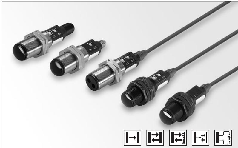
The 7000 series consists of a self-contained transmitter SMT, and a receiver SMR which are to be used in thru-beam mode, an SMP for diffuse proximity, SMRR for retro reflective and an SMPF for use with fibre optic cables. All are offered with sensitivity adjustment via integral potentiometer with either cable or plug connection.
