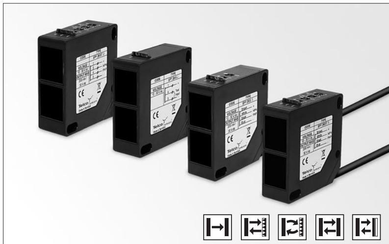
The SP 2000 series consists of a self-contained transmitter SPT and receiver SPR, which are to be used in thru-beam mode, SPRR for retro-reflective, SPPR for polarised retro-reflective, an SPP for diffuse proximity and SPBS for background suppression. All are offered with sensitivity adjustment via integral potentiometer with either cable or 180° rotatable plug connection.
