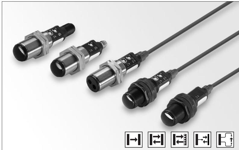
The 8000 series consists of a self-contained transmitter SMT, and a receiver SMR which are to be used in thru-beam mode, an SMP for diffuse proximity, SMRR for retro reflective and an SMPF for use with fibre optic cables. All are offered with sensitivity adjustment via integral potentiometer with either cable or plug connection.
