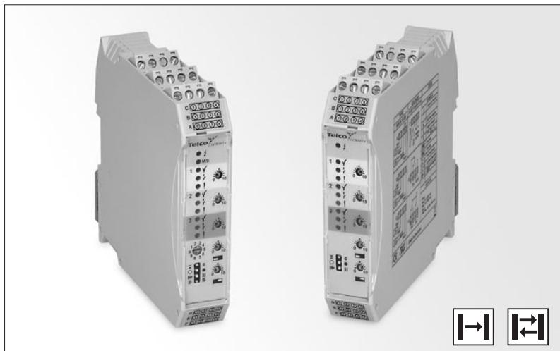
The PAB 30 is a 3-channel, multiplexed, photoelectric amplifier, which is to be used in conjunction with 3 sets of remote transmitters LT and receivers LR from the series 100, 110 and 120. The 3 channels operate independently of each other with their own set of remote transmitter and receiver. The multiplexing function ensures that optical cross talk between channels is prevented.
